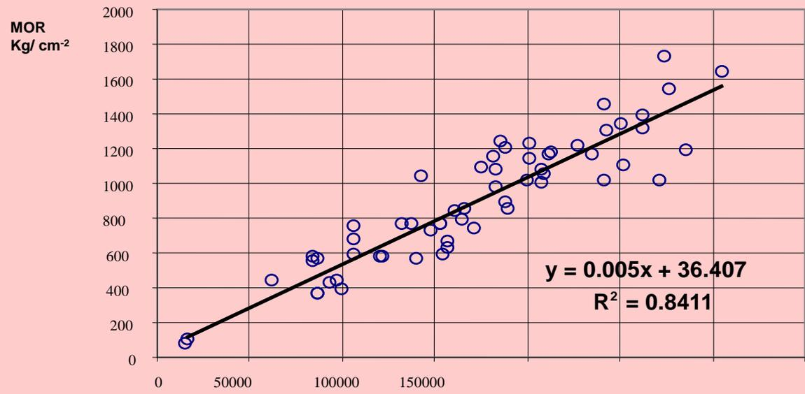
Figure 4. MOR (Static Bending) vs. MOE (Microsecond Timer)
