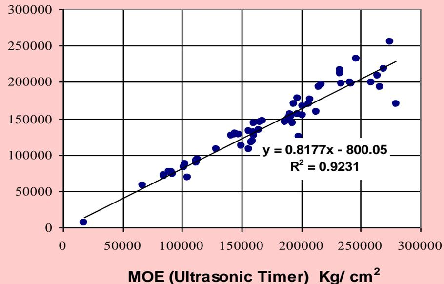
**Figure2.** Destructive method MOE (Static bending test) vs. Longitudinal MOE (Ultrasonic Timer)
