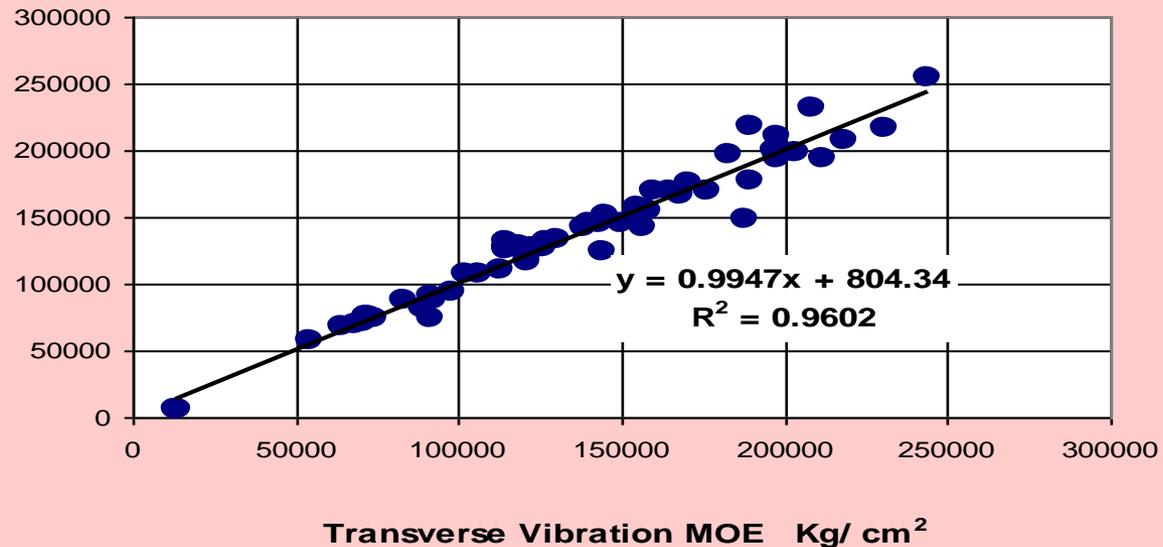
**Figure 3.** Static Bending MOE vs. Transverse vibration method MOE
