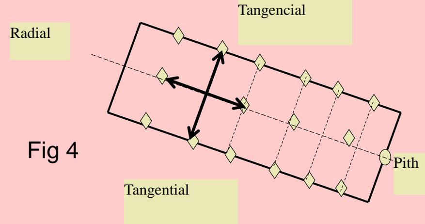
**Second way: Localization of points for angular measurement**
